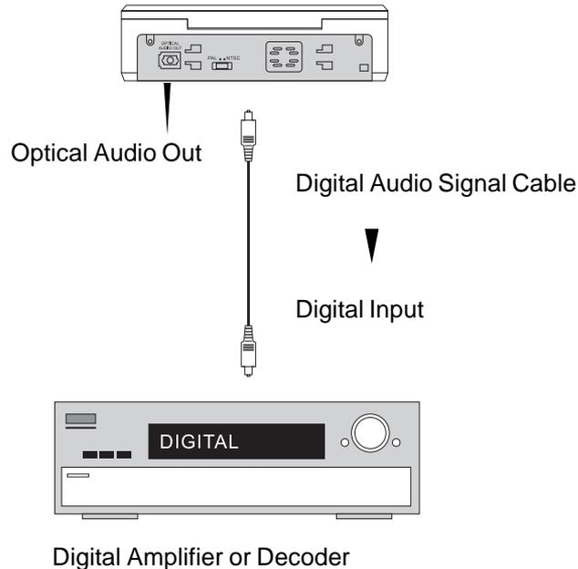
The audio portion of program discs can be output through the player's digital signal output port using the digital audio signal cable that is supplied with your player.
